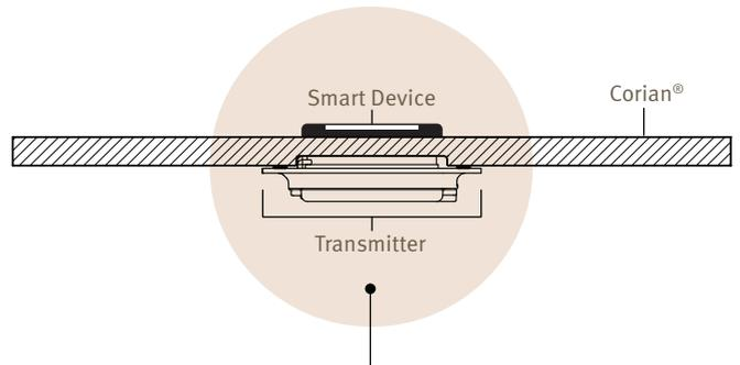
Hidden from view is a transmitter that powers up smartphones and tablets wirelessly.
