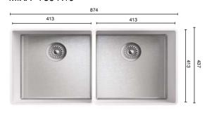
□ min. 900 mm Depth: 205 mm  $\bullet \bullet \circ$
