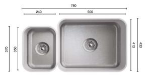
$_{\square}$  min. 900 mm  $\bigcirc$   $\bigcirc$   $\bigcirc$  Depth: 135 mm (L) and 200 mm (R)
